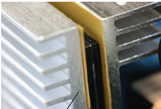
Figure 6: Thermal interface material bonding battery component to heat sinks.
