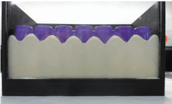
Figure 7: Foam encapsulating battery cells inside a battery module. Foams can be used to support and protect battery cells and may also slow or stop the spread of fire if there is a problem with the battery.
