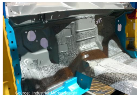
Adhesives and sealants on firewall and floor of steel pickup truck cab
