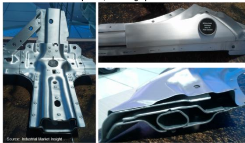
Ford F-150 aluminum pillars, showing spot welds and rivets
