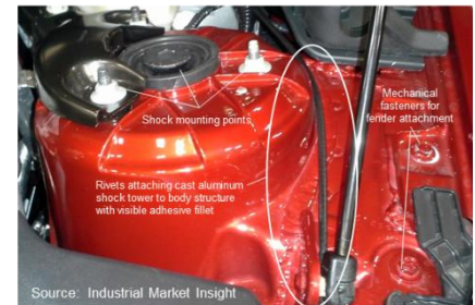
Aluminum shock tower joined to steel body rail with rivets and adhesives in Cadillac ATS
