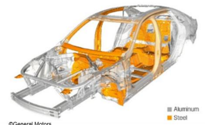
CADILLAC CT6 MIXED-MATERIAL STRUCTURE
