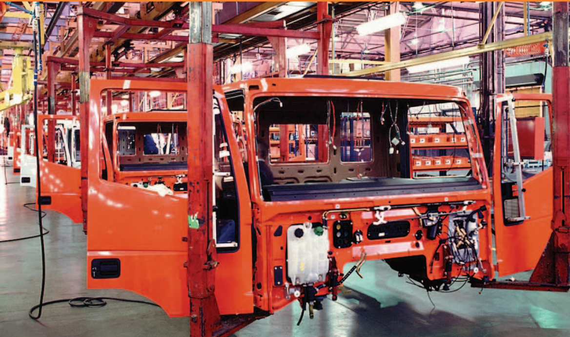
Figure 16: A heavy-duty truck cab in production.
