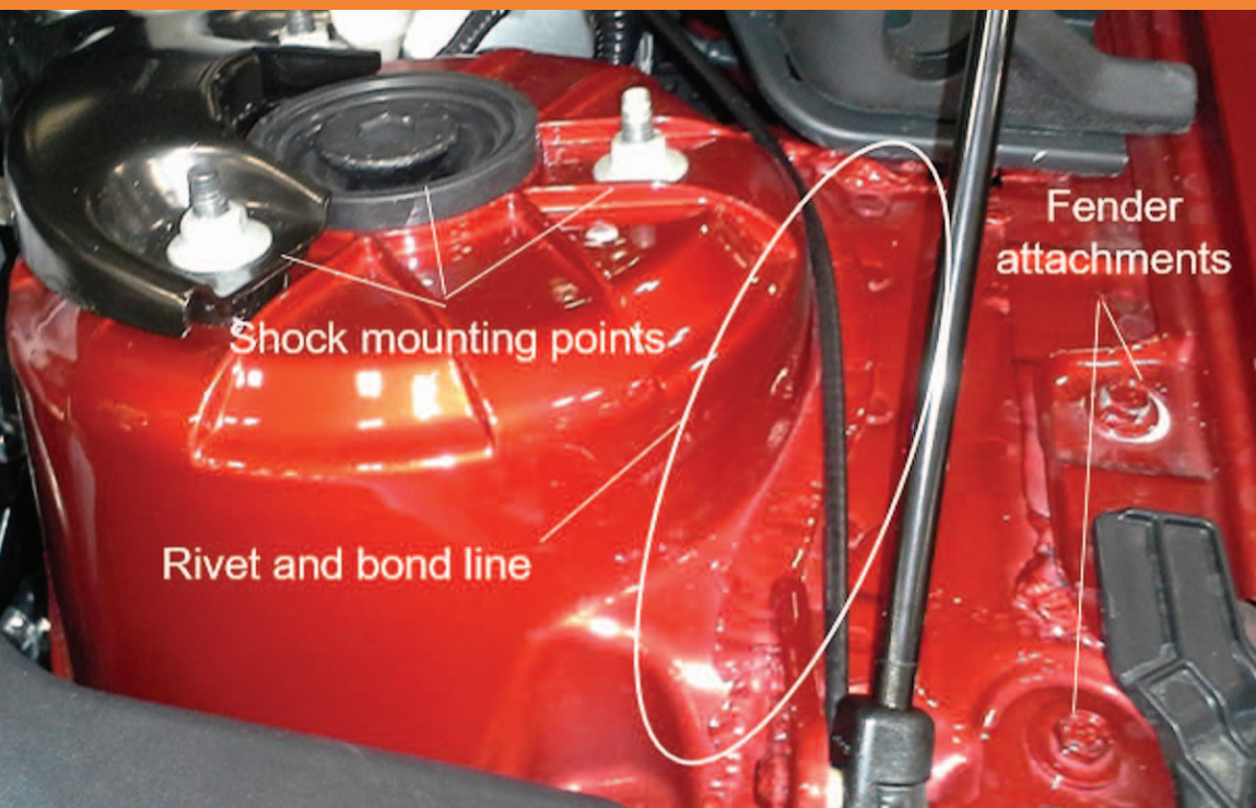
Figure 9: Cast aluminum shock tower rivet bonded to steel body in a vehicle. The location of rivets and the bond seam can be seen in the white oval in the photograph. Bolts attaching the strut, which is the top of the shock assembly, can be seen, as can the bolts attaching the fender to the body. Source: Industrial Market Insight
