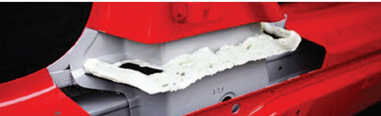
Figure 21: Cutaway showing location of preformed expanding foam sealant at the intersection of a frame rail and pillar. Expanding foams keep sound and moisture from moving through the white body and entering the cabin. Source: Sika
