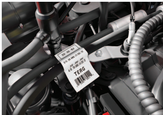
Figure 13: Wire harness label used for work-in-progress (WIP) tracking and identification. Source: Avery Dennison
