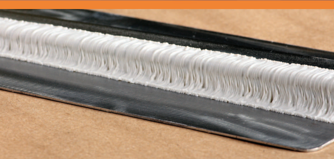
Figure 2: Paint sealer applied to a test section. The plastisol is streamed/swirled across the joint applied by a robot. The joint would be a non-cosmetic and does not require tooling after application. Source: Henkel
