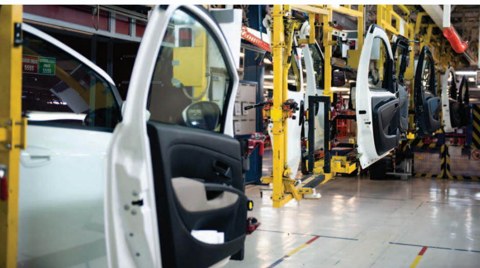
Figure 11: Door inner trim panel installed after moisture barrier.
