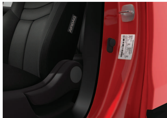
Figure 14: Door jam (B pillar) label with vehicle manufacturing details and VIN number. Source: Avery Dennison
