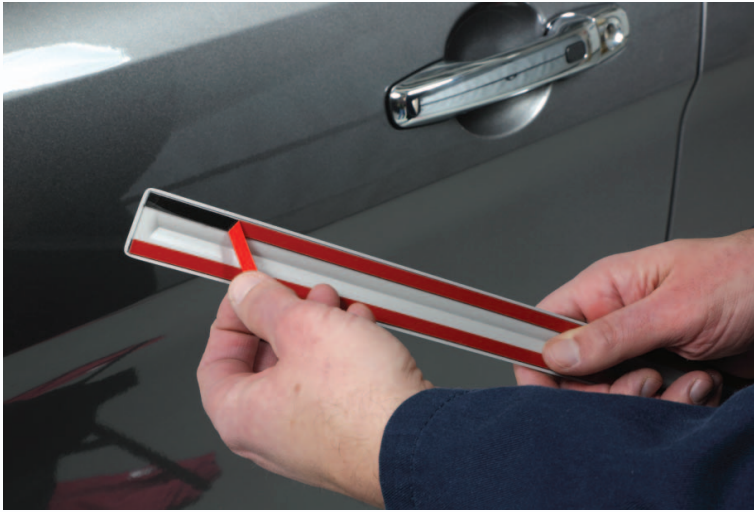
Figure 15: Moldings bonded with PSA. Source: 3M
