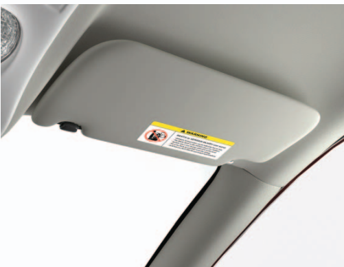
Figure 12: Visor warning label with car seat cautions. Source: Avery Dennison
