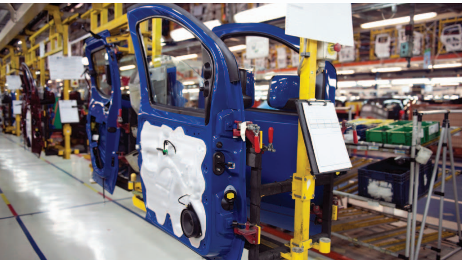
Figure 10: Door inner water shield bonded with a hot melt pre-applied PSA. The hot melt is robotically applied to die-cut plastic sheets to bond and seal the sheet before the door inner trim panel is assembled to the door.
