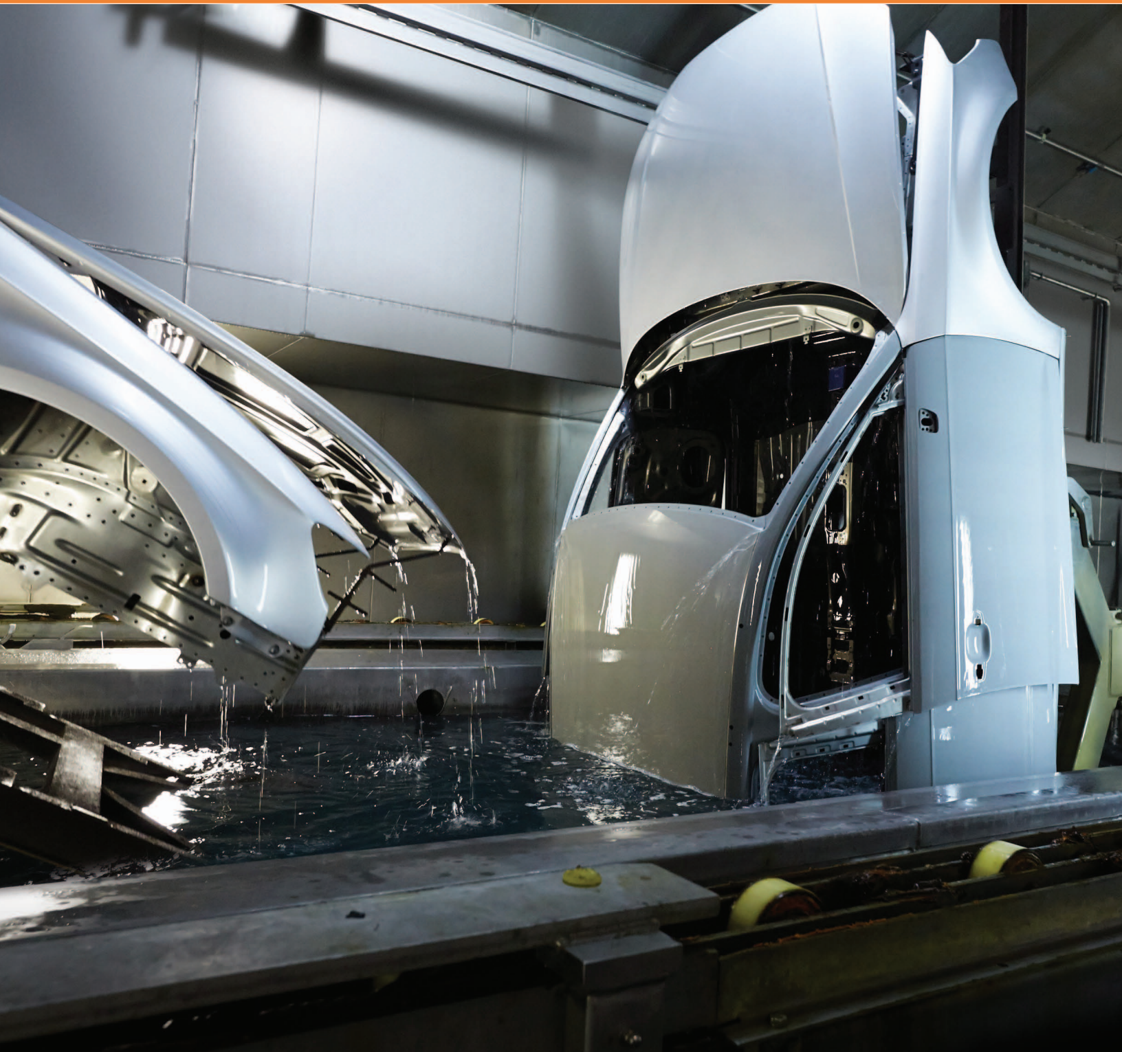
Figure 1: Car entering an automotive pre-treatment bath prior to ecoat. Car bodies are fully immersed in several wash, treatment, and rinsing baths before the adhesives and sealants applied in the body shop are cured in the e-coat oven. This is where the ASC Body Shop Guide Ends and where this guide picks up the process. Source: Henkel
